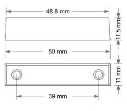
All dimension are in mm tolerance ±0.2mm
